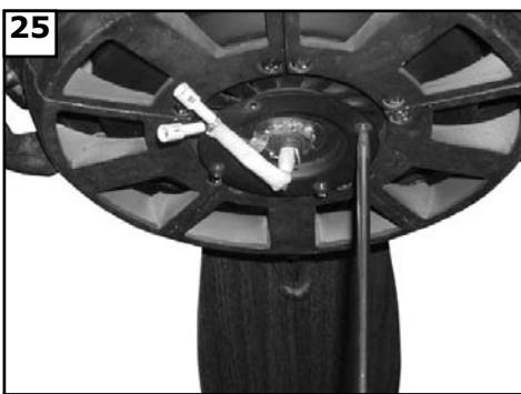
Loosen 3 screws with key slots and remove the screw without key slot.
